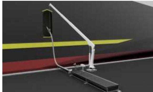
The LNG bunkering arm manages the transfer of fuel from shore to ship.
