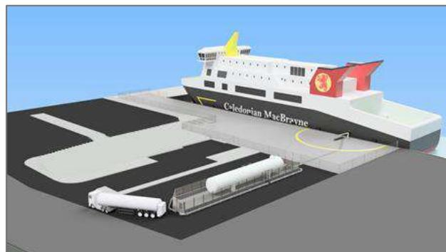
The LNG refilling of the shore based LNG tank will be managed by means of a transfer of fuel from road trailer to the static holding tank.
