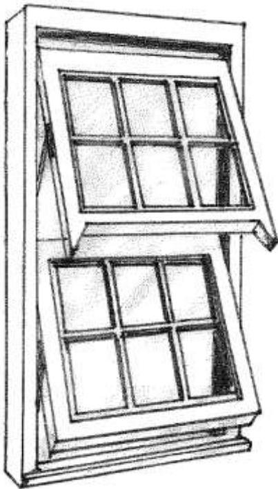
Most modern tilting sash windows are reversible to allow cleaning from inside.
